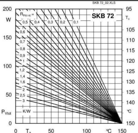
Fig. 3R Power dissipation vs. case temperature
