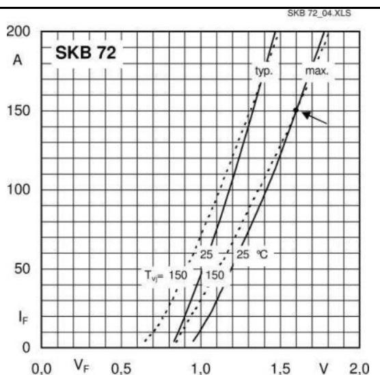
Fig. 9 Forward characteristics of a diode arm
