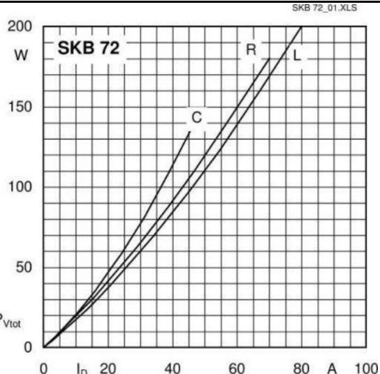
Fig. 3L Power dissipation vs. output current
